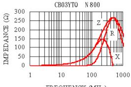
FREQUENCY (MHz) RDC: 0.4 Ω Rated current:300 m A
