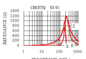
FREQUENCY (MHz) RDC: 0.5 Ω Rated current:200 mA
